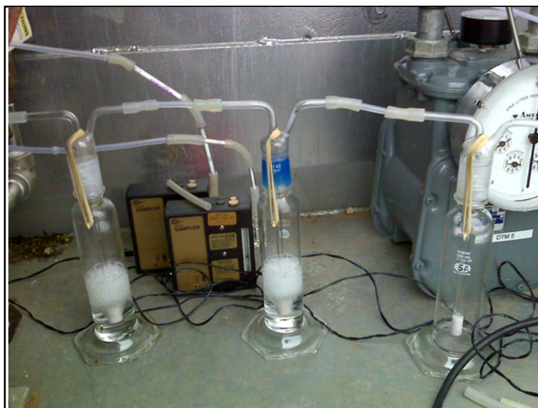
Figure 43: Impinger Train of \text{HNO}_3/\text{H}_2\text{O}_2 Solution.
