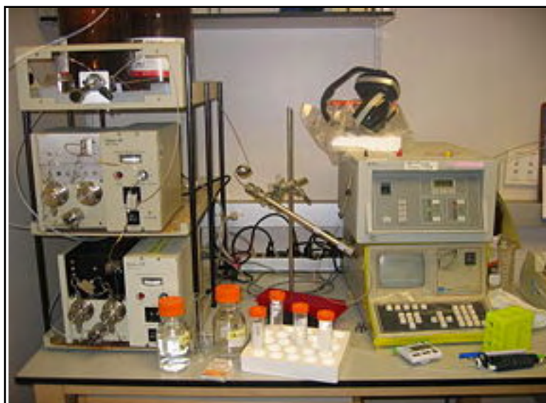
Figure 39: A High Performance Liquid Chromatography Unit. From left to right: HPLC pump, steel-reinforced column, apparatus for measuring absorbance.
