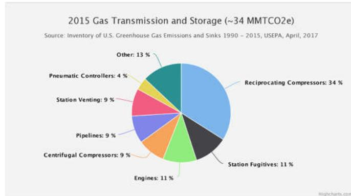
**Figure 5. Methane Emissions from Gas Transmission and Storage**
