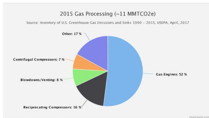
**Figure 4. Methane Emissions from Gas Processing**
