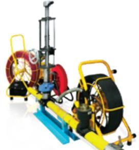
Marketed as the Kleiss MCS Flow Stopping System, new tools are used to stop the flow of gas in polyethylene, steel, cast-iron, and PVC pipes at diameters up to 18 inches and pressures up to 60 psig. The system, which is manufactured in Europe, was brought to the U.S. and optimized for North American infrastructure through an OTD project.
