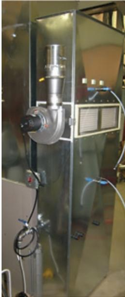
GTI's patented Transport Membrane Condenser (TMC) technology is a low-temperature device that recovers both sensible and latent waste heat and clean water from exhaust flue gas in industrial and commercial boilers. The technology has also been proven in residential markets, where the **Transport Membrane Humidifier (TMH) can simultaneously upgrade mid-efficiency furnaces (80%) to high-efficiency (95%) while also providing space humidification without an external water supply.**
