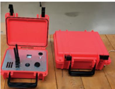
Another new tool simultaneously measures CH<sub>4</sub> concentration, air flow, temperature, and humidity for improved measurement and quantification of leak classification.
