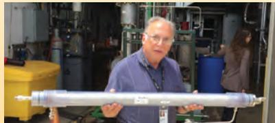
CarboLock has been shown to capture equivalent amounts of CO<sub>2</sub> with less than 10% of the volume required by conventional gas/liquid contacting equipment in slipstream testing at a coal-fired power plant in Illinois.
