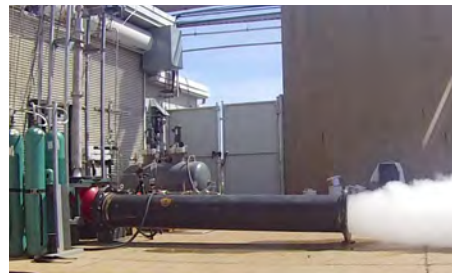
Steam generator with lime slurry injection for CO 2 separation. Exhaust stream is steam and reduced CO 2 .
