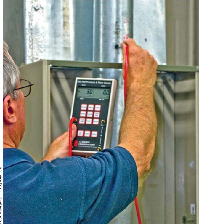
**Fig. 5.11 Measuring exhaust vent draft suction**
