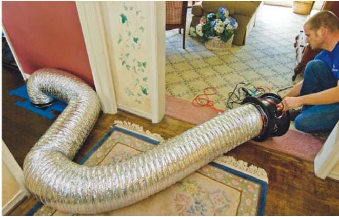
**Fig. 3.10 - Measuring duct tightness**
