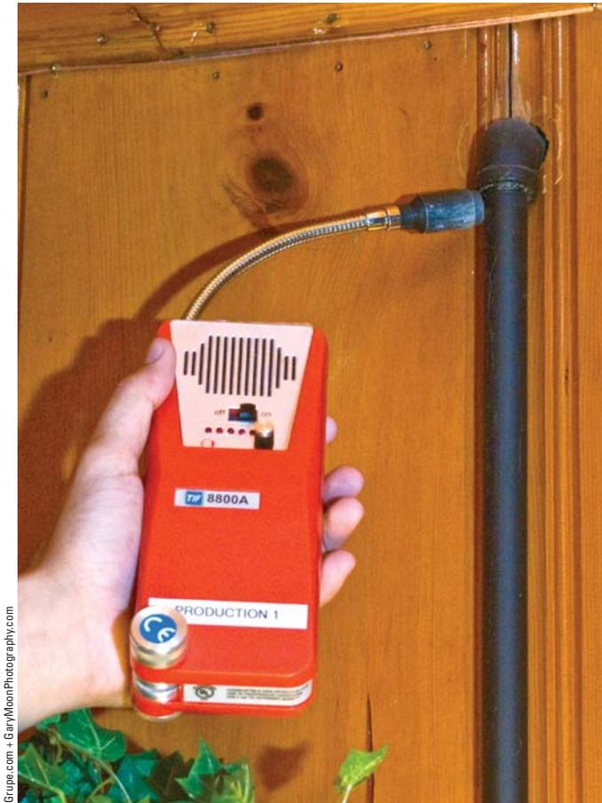
Fig. 5.13 Electronic gas leak detector - Audible indicator
