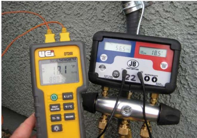
**Fig. 5.21 Semi-automatic superheat and subcooling calculations**
