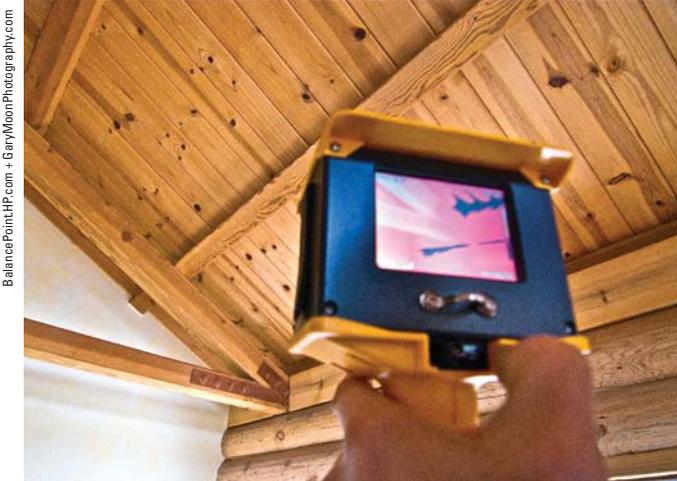
**Fig. 9.15****Thermal cameras can help locate less-obvious air leakage points**
