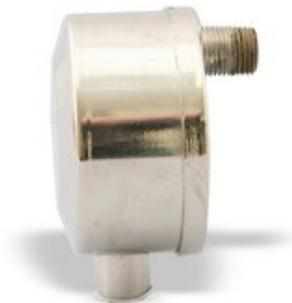
**Figure 6. Gorton No. 4 angle radiator vent. Gorton models are made in No. 4, 5, 6, C, and D, ranging from 4 with the smallest orifice (for warm apartments) to D with the largest (for cool apartments)**
