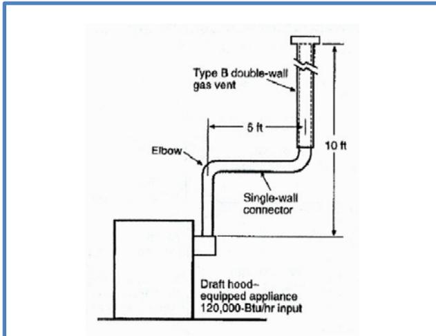
**Figure 1. Draft hood-equipped appliance**
