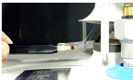
**Figure 8. Draft hood-equipped water heater smoke pen testing**
