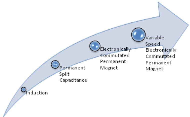
**Figure 1. Electric motor options by increasing efficiency**
