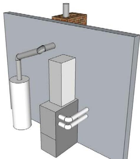
**Figure 4. After replacement; note the chimney liner**
