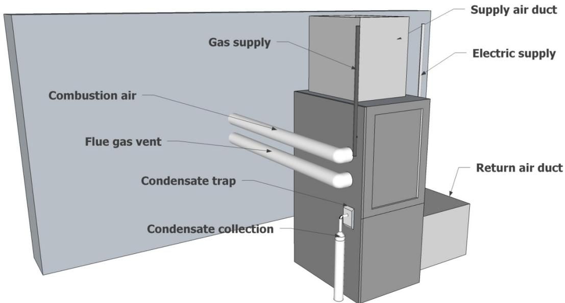
**Figure 7. High efficiency furnace components**
