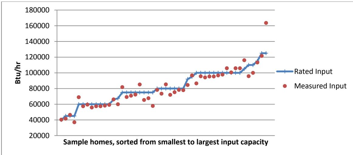
Figure 6. Btu/h input to furnace
