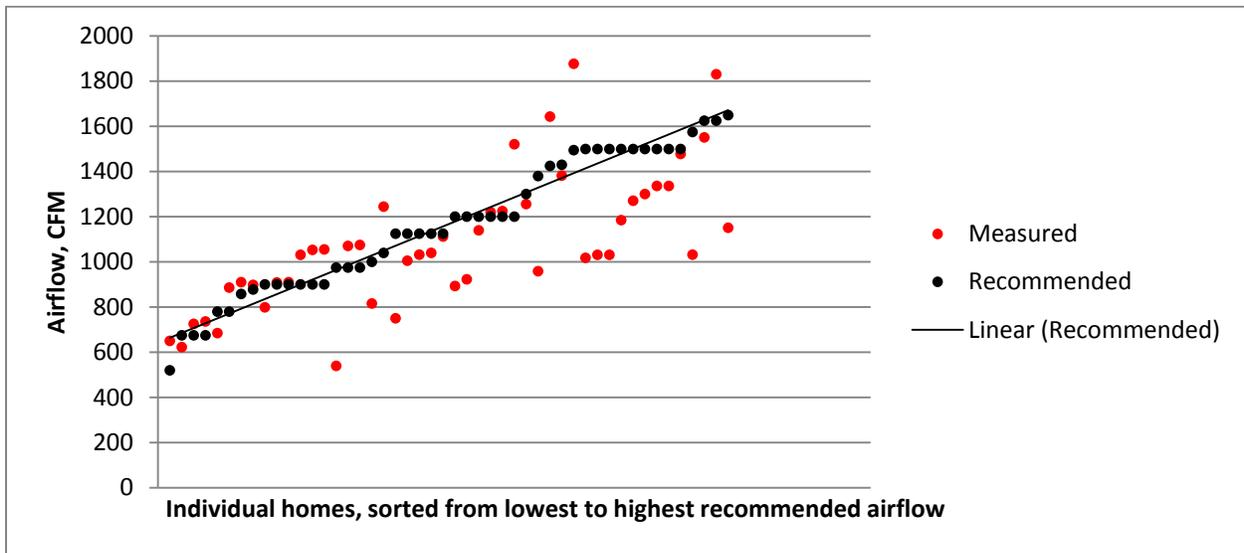
Figure 3. Recommended and measured airflows by individual home
