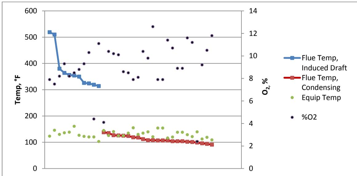
Figure 7. Results of flue gas testing (Condensing and Induced draft furnaces)
