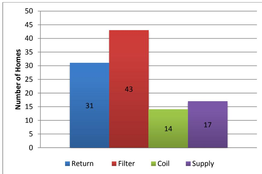
**Figure 21. ESP restriction, by location**
