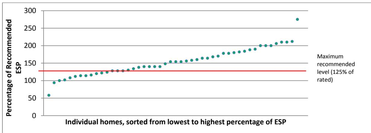
**Figure 20. Percentage of required airflow across heat exchanger as measured in the home**
