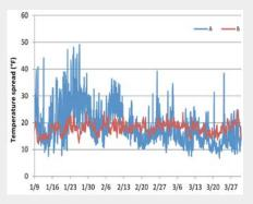
High resolution temperature data were collected at two test buildings. The graph shows a wide range of temperatures and spreads among units and over time.
