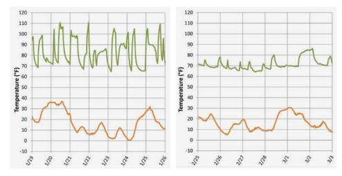
Left: pre-retrofit. Right: post-retrofit. The extreme temperature peaks in the test building decreased significantly, which probably indicates that ovens were used much less for heating. (Green lines indicate unit temperature.)
