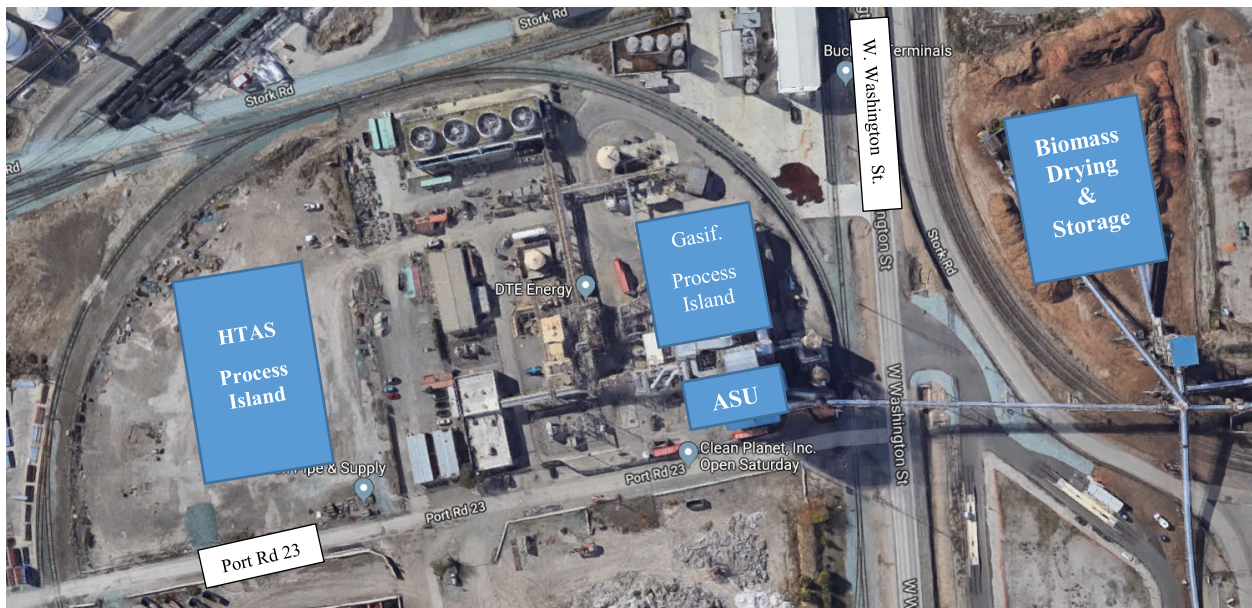
Figure 7. Layout of the New Process Islands and Biomass Drying/Storage
